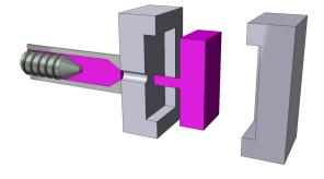
The moving platen, or B-side, of an injection molding machine is moved by a hydraulic ram or mechanical toggle on a hydraulic or electric molding machine.
