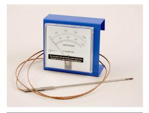
A pyrometer is a type of thermometer that is used to measure high temperatures.
