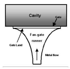
The fan gate helps prevent warping of parts by reducing strress concentrations in the gate area.
