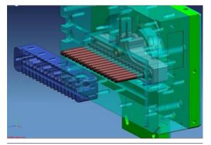
A hot-runner mold is insulated and kept hot in order to produce parts without scrap.
