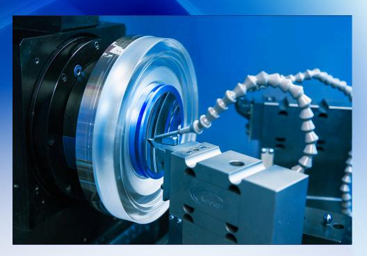
**Single Point Diamond Turning (SPDT):** A Singular Solution for Precise Optics Prototyping
