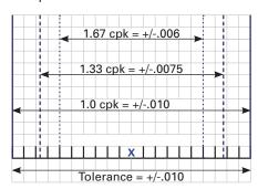
Gauge repeatability (Gauge R&R) determines how much of the tolerance is lost to measurement variation.
