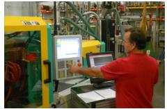
Scientific molding, as used by Empire Precision Plastics, is a recognized method for improving the quality of injected molded parts and assemblies. This approach identifies and controls key processing factors such as temperature and cavity pressure to ensure consistently high quality from operator to operator, shift to shift and part to part.
